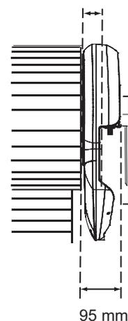
Ensure that there is at least 45 mm from the edge of the curtain to the edge of the bracket. If the roller door drum wheel is on the edge of the curtain or is a smaller diameter, additional clearance may be required.
